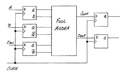
The sum and carry out networks can be realized in two level sum of products representation and can be implemented with either AND and OR gates, or with NAND gates alone. In either case inverters aren't necessary since the input D flip flops provide both the true and complemented versions of A, B and Cin.
